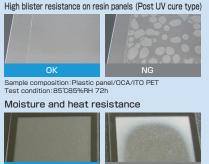
Sample composition: Plastic panel/OCA/Glass Test condition: 85°C85%RH 120h
